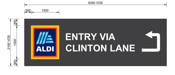
SIGN 1 ALUMINIUM SUB FRAME WITH BACK BOARD WITH DIGITALLY PRINTED FLEXFACE MECHANICALLY FIXED TO EXISTING WALL. NON ILLUMINATED WITH ANTI GRAFFITI COAT.
